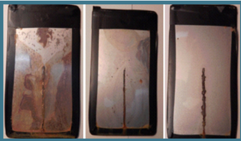
FIG C CORROSION RESISTANCE SALT SPRAY ASTM B 117-09 1056 HRS.
